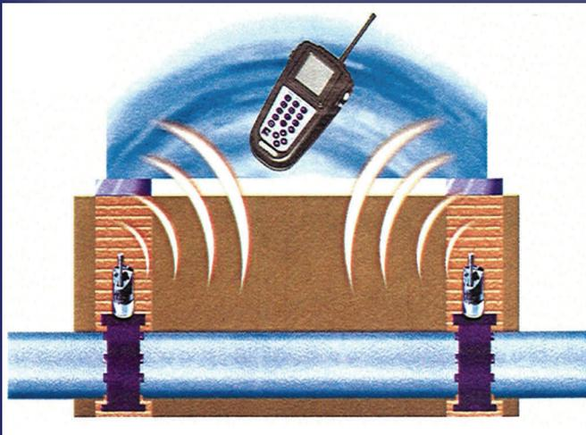
**Leak Detection System.** Magnetized Units transmit leak status signals to Patroller unit
